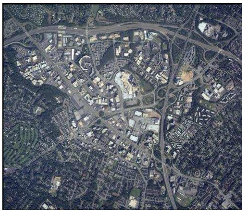
Figure 10 - “Tyson's Corner” This aerial photo, taken in Virginia around 2007, shows low-density development shaped by separate-use zoning codes and a street system featuring freeways, arterials, collectors and cul-de-sacs instead of an urban grid network. Source: http://www.cnu.org/node/1333
